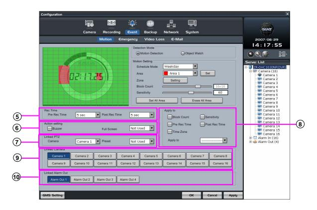
**Zone** : Set the time period for which each area setup will be used. In the zone setting select the schedule mode and then select the area to set over the 24hr time line period.
